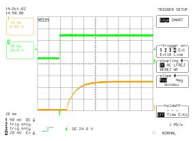
iHA48060A012V-001 Typical startup characteristic from input voltage application at full load. Upper trace-input voltage, lower trace – output voltage
